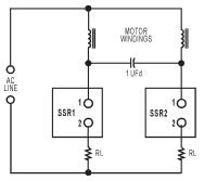
The resistors are unnecessary if the control circuit is designed to ensure one SSR is off before the other SSR is on.
