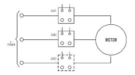
Three-phase motors may be controlled by solid-state relays as shown. A third SSR as shown is optional, but not necessary. The control windings may be connected in series or parallel. Care should be taken to ensure that surge current drawn by the motor does not exceed surge current rating of the SSR.
